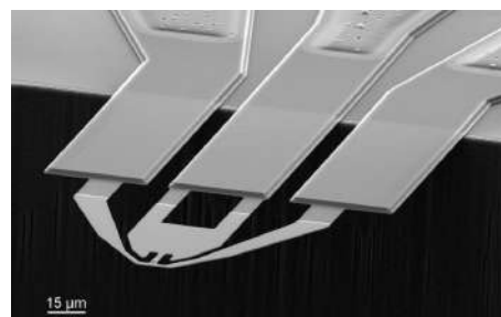
NanoFrazor Cantilever made of Si
